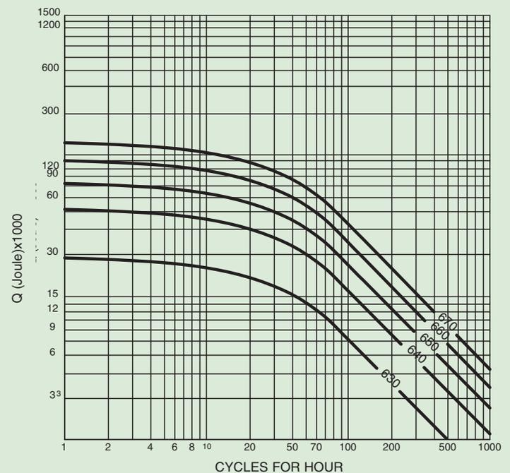
The cooling rates represented by the above curves are based on an external lubricant flow of 4 liters per minute through the disc pack
