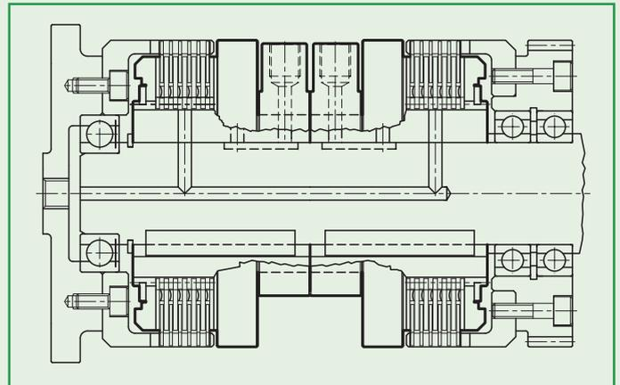
**Back to back duplex arrangement with integral oil collector**
